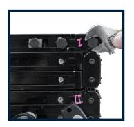
Remove the three bolts already in place at the top and bottom edges of the main panels.
